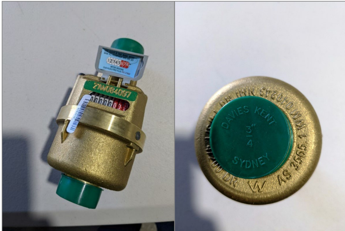
Figure B.2.1 Potable water meter; Australian Standard and NMI compliance embossed on body of meter.
